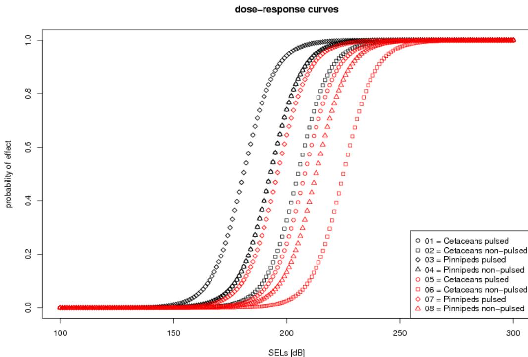
**Figure 1: Dose-response curves used within SAFESIMM to relate the probability of Temporary Threshold Shift (black curves) and Permanent Threshold Shift (red curves) to M-weighted Sound Exposure Level (SEL) for cetaceans and pinnipeds exposed to pulsed and non-pulsed sounds.**
