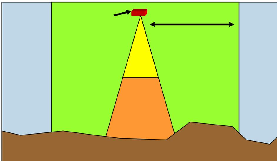
**Figure 5 : Schematic diagram of modelling zones for an air-gun array. Zones 1 & 2 contain the main downward propagation beam. Within zones 1, 2 & 3 spherical spreading can be assumed. Absorption and bottom effects are also low so propagation is frequency independent.**
