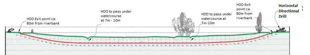
Fig. 4 Typical HDD Cross Section
