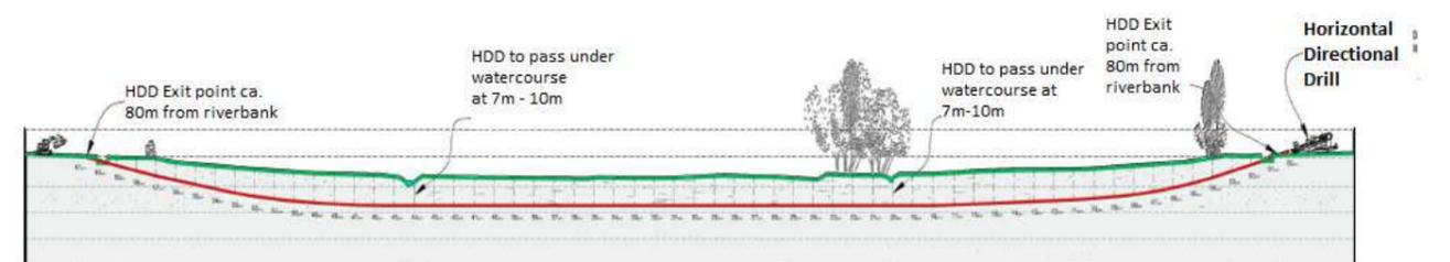
Fig. 4 Typical HDD Cross Section
