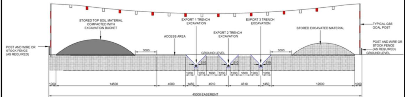
Fig. 3 Typical Easement Cross Section
