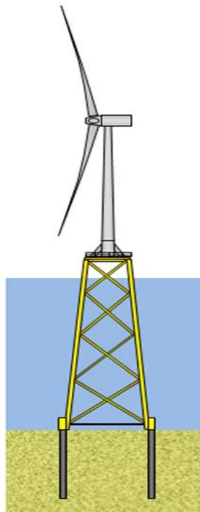
**Figure A.2. Outline Design of the Proposed Jacket on Pin Pile Foundation**
