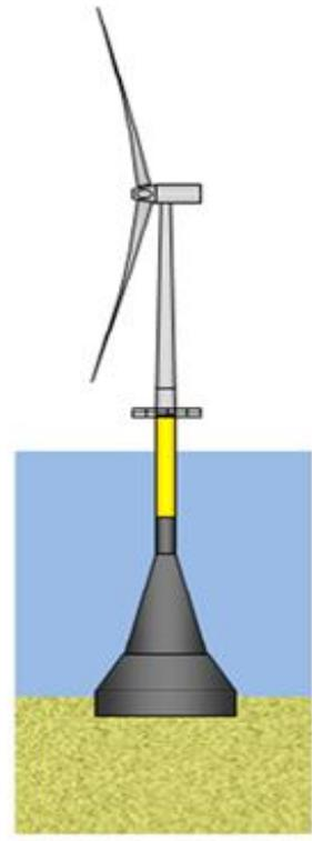
**Figure A.1. Outline Design of the Proposed Gravity Base Foundation**
