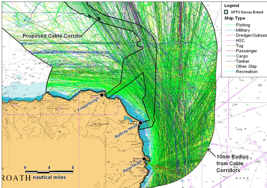
**Figure 5.4 Ivero Survey Southern Section of Cable Route (28 Days AIS tracks)**
