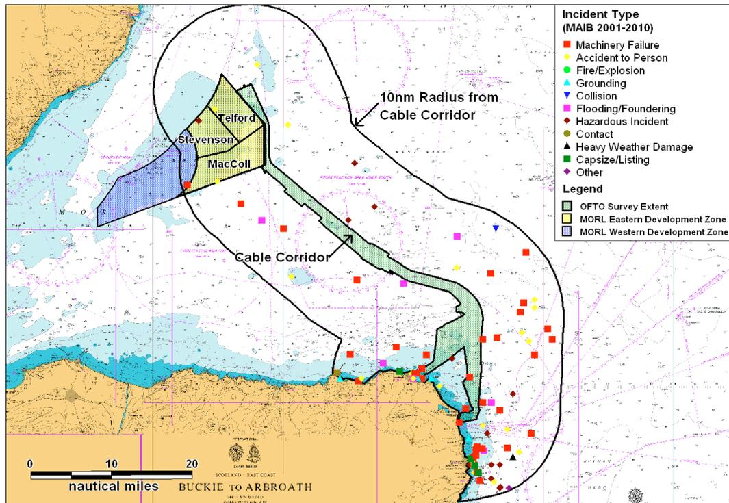
**Figure 4.1 MAIB Incident Locations by Type within 10nm of Cable Route**
