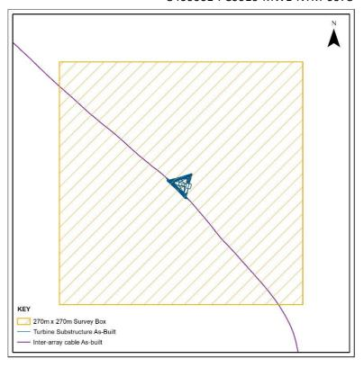
Figure 2: Survey area around each WTG – example
