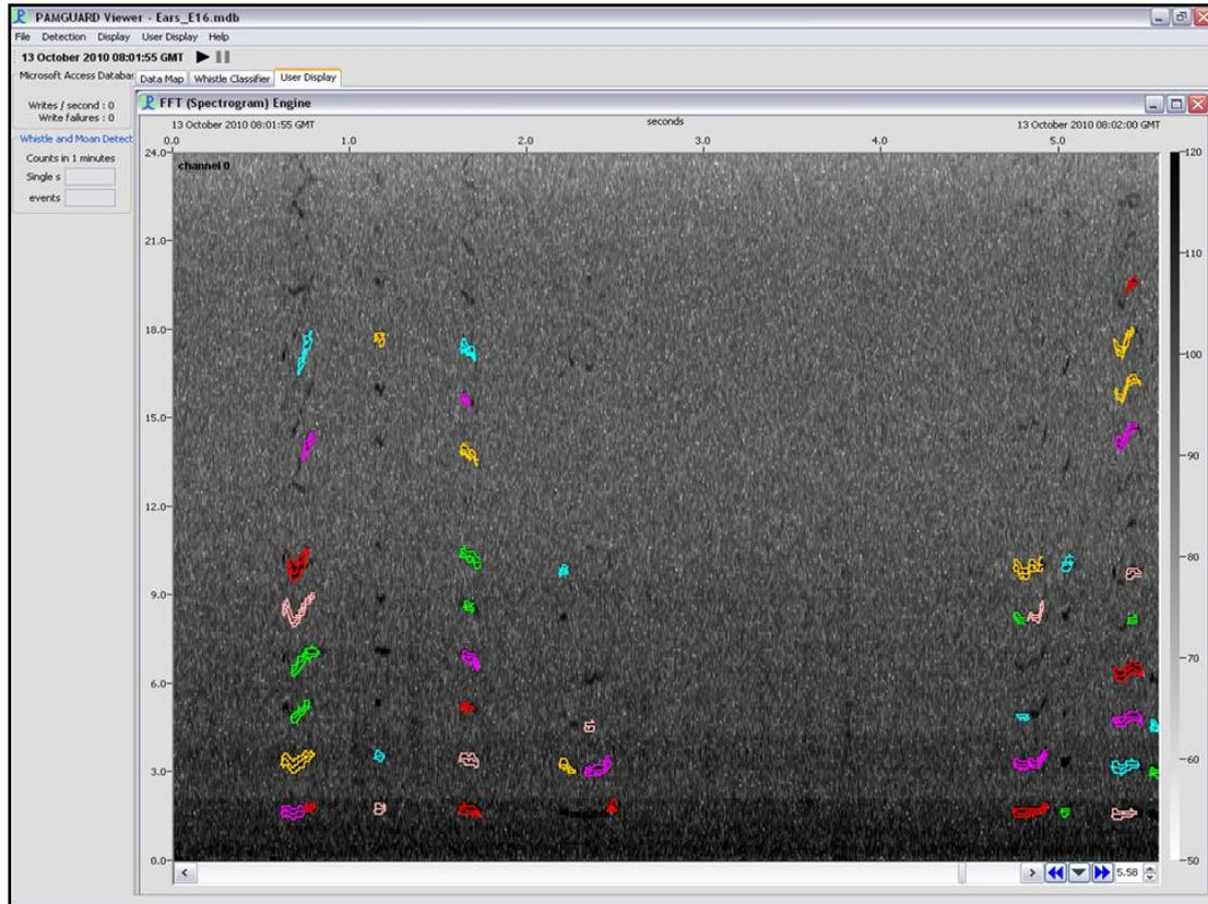
**Figure 7.8: Screenshot from PAMGUARD whistle classifier of a 'rubbing' false detection. Frequency is on the y-axis and time (5.58 seconds) is on the x-axis. The different colours show the contours generated by the WMD.**
