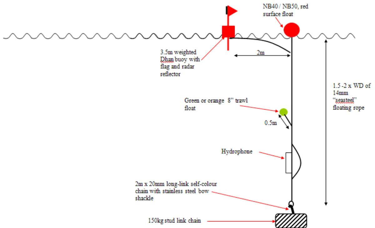
**Figure 5.14: Single riser mooring design with Dhan buoy used to suspend PoDs in the water column.**
