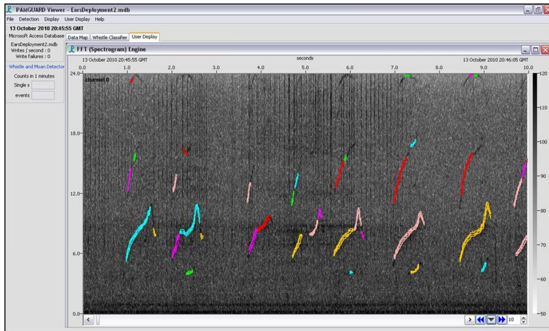
**Figure 7.4: Example screen grab showing whistle contours extracted from recordings of bottlenose dolphins using PAMGUARD. Frequency (kHz) is on the y-axis and time (10 seconds) is on the x-axis). The different colours show the contours identified by the WMD (clicks are also visible above 6 kHz).**
