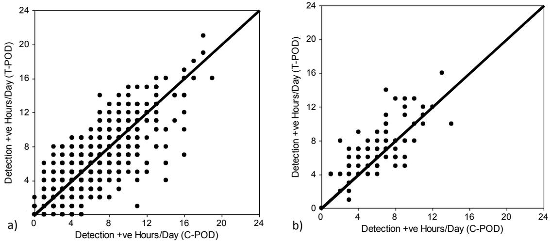
**Figure 5.32: Comparison of the number of hours per day that porpoises were detected on paired T-PODs and C-PODs in 2010; a) for all nine paired devices (see Table 5.12) and b) data for the Beatrice Demonstrator site. The line shown on each figure represents a 1:1 relationship.**
