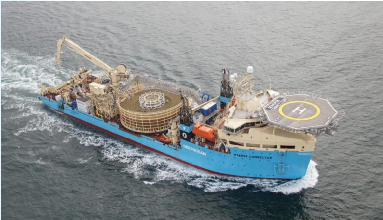
Figure 4-1: Example CLV which could be used to recover the interconnector cables. The large cable carousel can be seen in the middle of the vessel.
