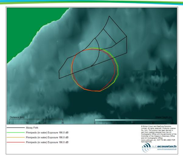
Figure 4.5: Comparison of maximum SELs for Pinnipeds in water (186 dB) based on one (red line), two (orange line) or four (green line) 2.5 m diameter pin piles being installed within a 24 hour period.
