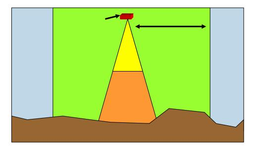
Figure 5 : Schematic diagram of modelling zones for an air-gun array. Zones 1 & 2 contain the main downward propagation beam. Within zones 1, 2 & 3 spherical spreading can be assumed. Absorption and bottom effects are also low so propagation is frequency independent.
