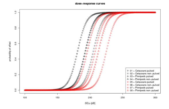
Figure 1: Dose-response curves used within SAFESIMM to relate the probability of Temporary Threshold Shift (black curves) and Permanent Threshold Shift (red curves) to M-weighted Sound Exposure Level (SEL) for cetaceans and pinnipeds exposed to pulsed and non-pulsed sounds.
