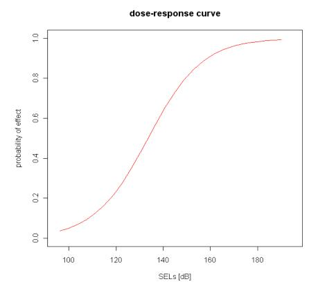
Figure 2. Dose-response curve used within SAFESIMM to relate the probability of behavioural displacement to M-weighted Sound Exposure Level (SEL) used for cetaceans and pinnipeds exposed to pile driving noise.
