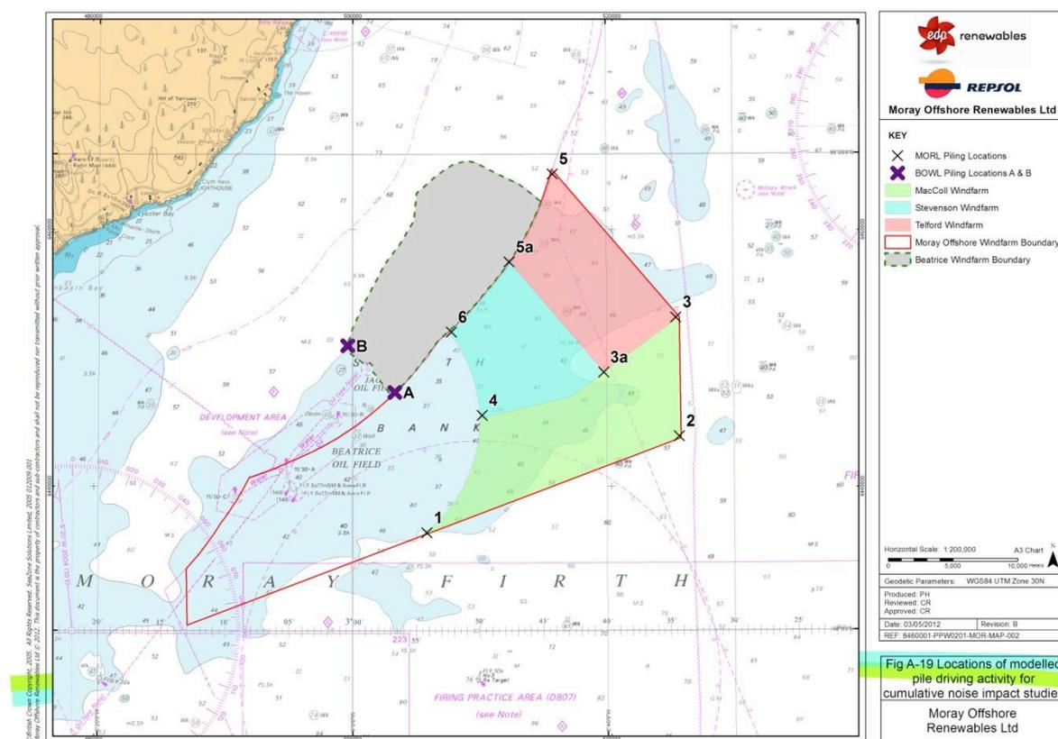
Figure A-19. Sketch map, showing locations of the piles whose driving has been modelled.
