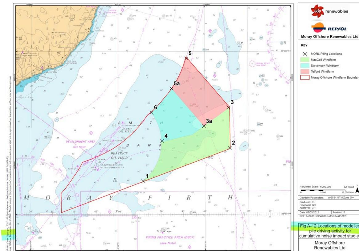
Figure A-12. Locations of modelled pile driving activity for scenarios 1, 2 and 3 above.
