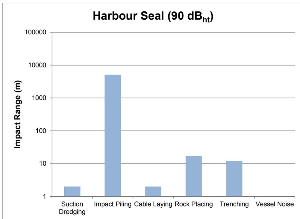
Figure A-8. SPEAR model to illustrate typical source noise associated with a range of construction related activities.
