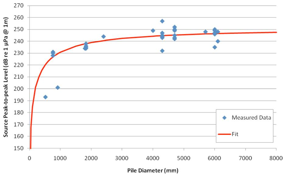
*Figure A-7. Plot showing the asymptotic best fit to Source Level calculated from measured piling noise data for various pile sizes*
