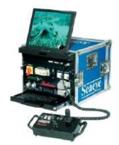
INPUT POWER REQUIREMENTS: Single phase universal auto sensing input, 100-270 VAC at 2.8 kW.
