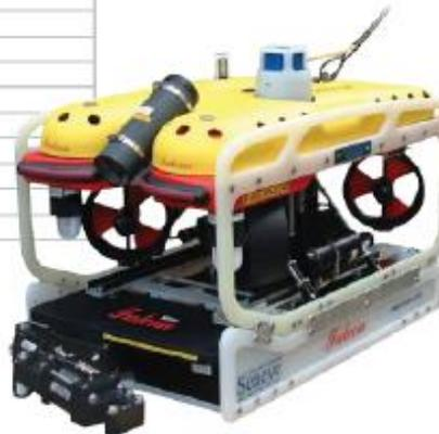
STANDARD FALCON WITH WIRE ROPE CUTTING SKID
